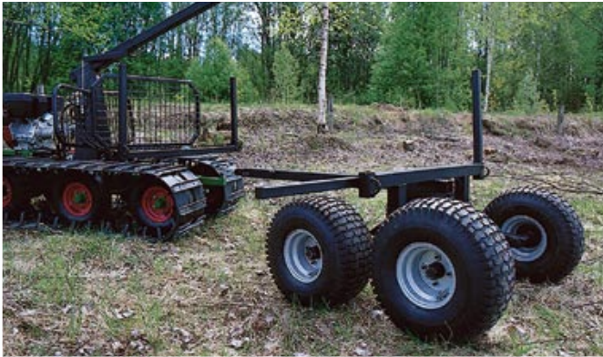
Oxen with bogie log trailer. Load capacity is approximately 1 cubic metre of solid wood. Oxen can also be equipped with a self-unloading timber cart.
