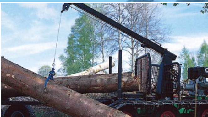
The log loading is easily done with the heavy duty loader crane and power winch. Lifting capacity is 300 kg.
