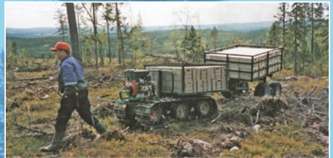
Oxen is equipped with a platform designed for transportation of plants.
